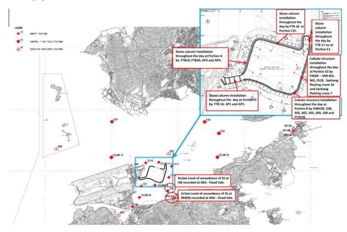
4.7.3.1 As informed by the Contractor, stone column installation was carried out throughout the day at Portion D by FTB 16, AP1 and AP2; at Portion A by FTB 19, FTB 20, AP3 and AP4; at Portion C2c by FTB 18 and at Portion E1 by FTB 17. Cellular structure installation works were conducted at Portion E2 by ES668 SHB 401, WK, ES18, Sanhang floating crane 16 and Sanhang floating crane 7 and at Portion B by SHB190, 208, 305, 402, 205, 209, 189 and FY3228.
