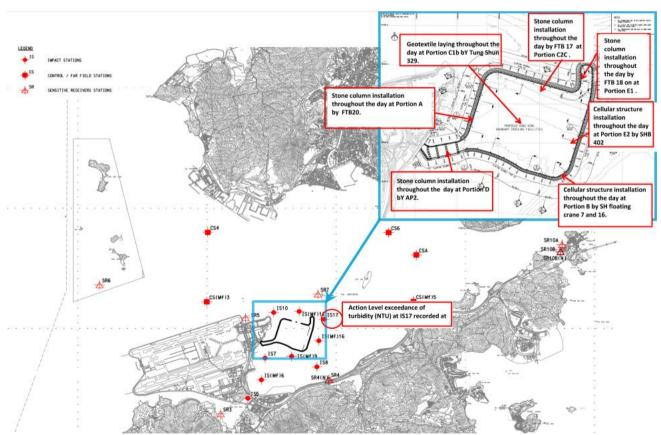
4.7.4.1 Stone column installation was carried out throughout the day at Portion D by AP2 and AP4; at Portion A by FTB 20; at Portion C2c by FTB 17 and at Portion E1 by FTB 18. Cellular structure installation works was conducted at Portion E2 by SHB 402; at Portion B by SH Floating Crane 7 and 16;
