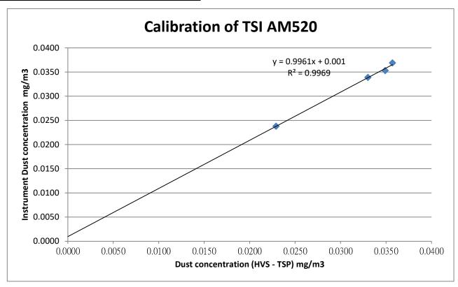
\*\*\* Filter paper being used in the calibration : 209591, 209592, 209593, 209594 Those filter papers are weighted by HOKLAS laboratory (ALS Technichem (HK) Pty Ltd.)
