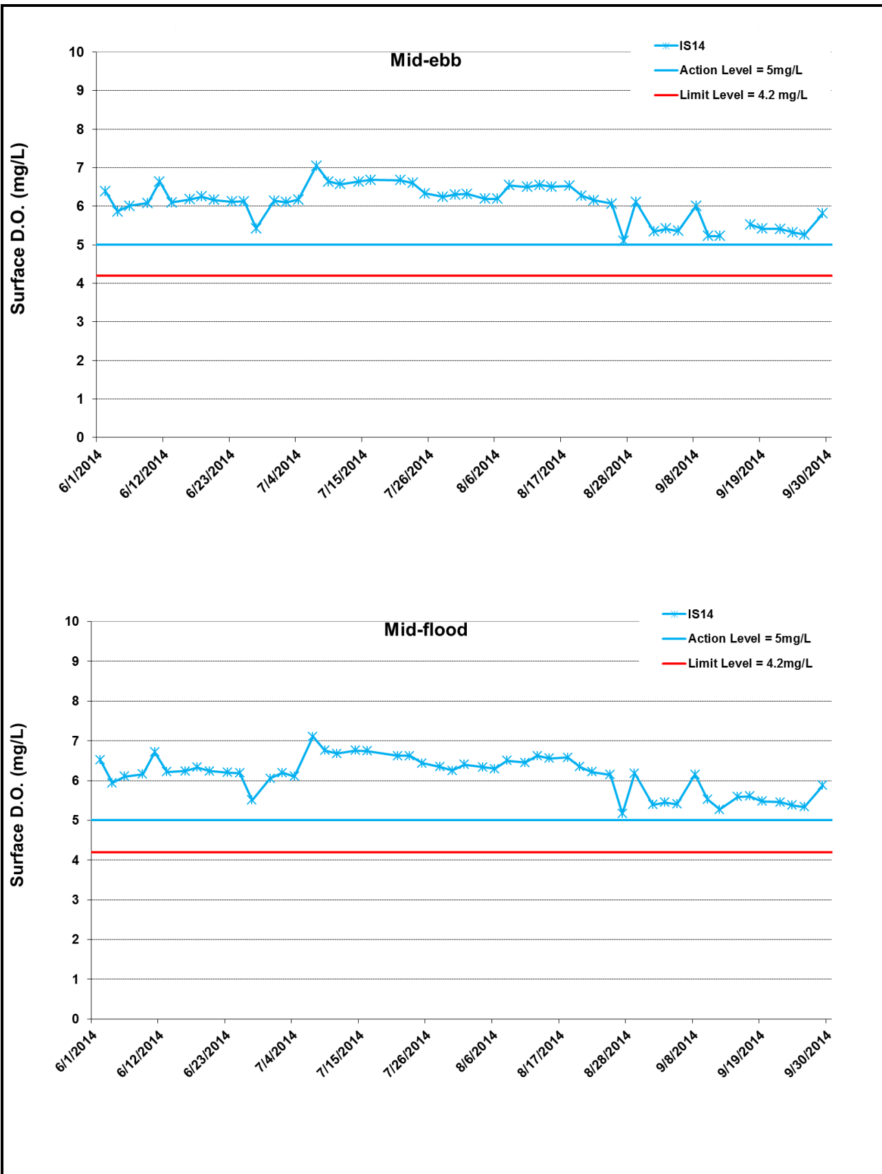
Figure I5 Impact Monitoring - Mean Level of Dissolved Oxygen (mg/L) in surface waters between 1 June 2014 and 30 September 2014 at IS14. The weather conditions during the monitoring period varied mostly from sunny to cloudy. Major marine construction activities included: Dredging (6/1/2014 - 8/6/2014); Construction of Temporary Seawalls (6/1/2013 - 9/30/2014); Sheet Piling (6/1/2014 - 9/30/2014); Filling (6/1/2014 - 9/30/2014). Please note WQM Mid-Ebb on 15-Sep was cancelled due to adverse weather.
