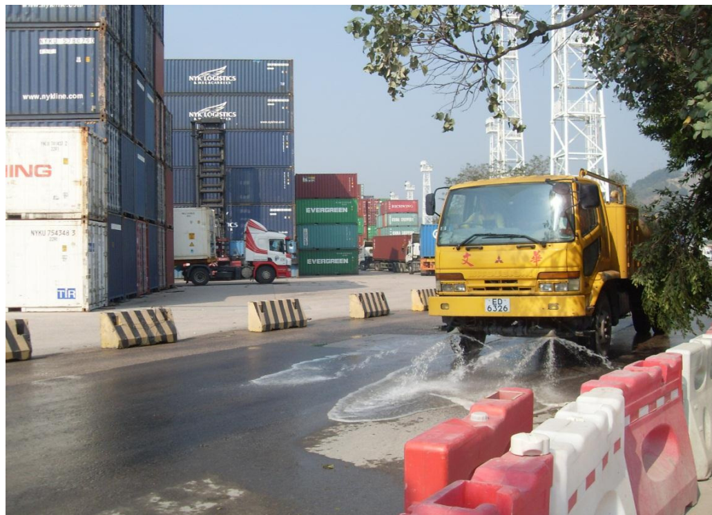
Water truck was observed in used during site investigation. (Haul road at River Trade Terminal)
