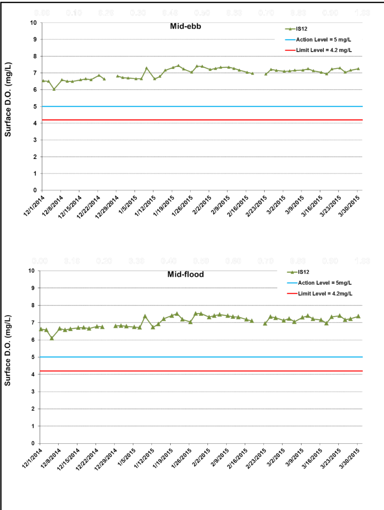
Figure I3 Impact Monitoring - Mean Level of Dissolved Oxygen (mg/L) in surface waters between 1 December 2014 and 31 March 2015 at IS12. The weather conditions during the monitoring period varied mostly from sunny to cloudy. Only minor marine works included rock bund deposition for marine sheet pile remedial works was carried out from 1 January 2015 to 28 February 2015. WQM on 20 February 2015 was postponed to 23 February 2015.
