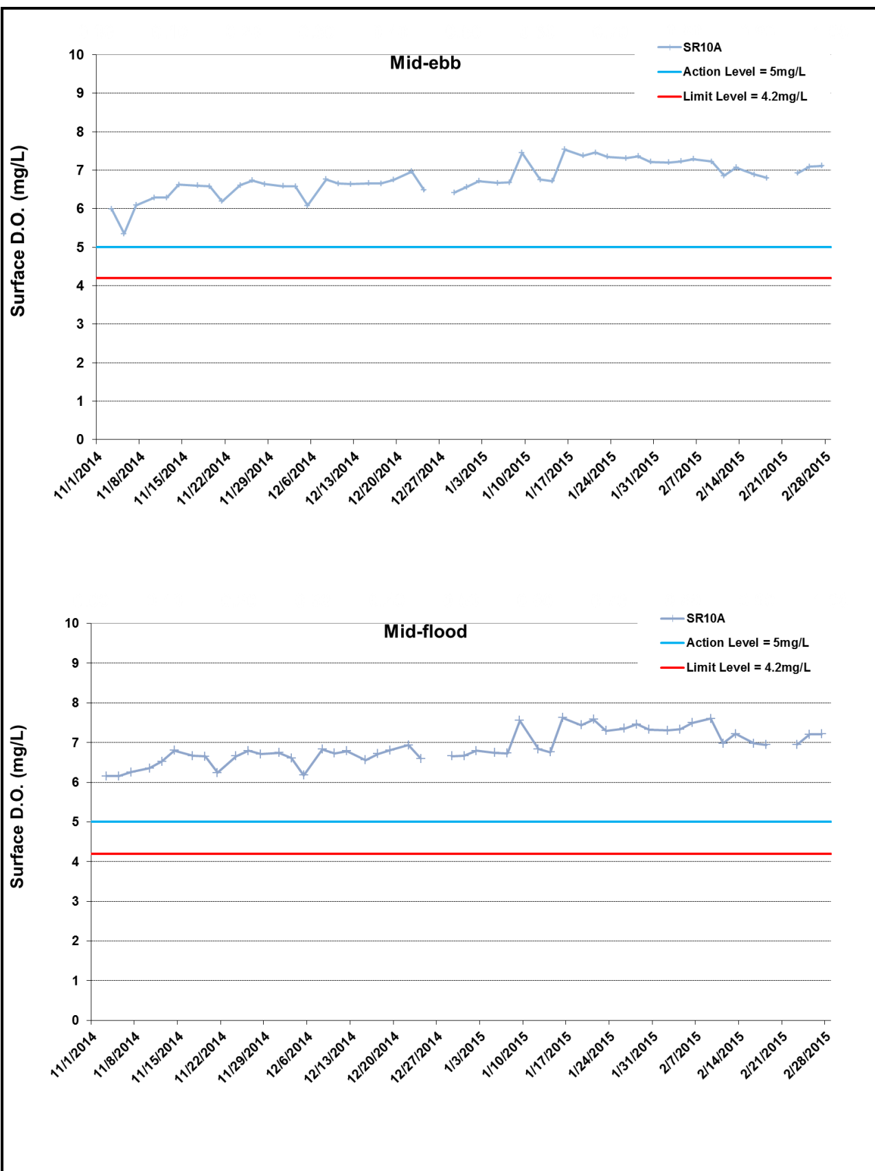
Figure G7 Impact Monitoring - Mean Level of Dissolved Oxygen (mg/L) in surface waters between 1 November 2014 and 28 February 2015 at SR10A. The weather conditions during the monitoring period varied mostly from sunny to cloudy. Major marine construction activities included: Construction of Temporary Seawalls (11/1/2014 - 11/20/2014); Sheet Piling (11/1/2014 - 11/20/2014); Filling (11/1/2014 - 11/20/2014). WQM on 20 February 2015 was postponed to 23 February 2015. Ref: 0212330_Impact-WQM_February2015_graphs_Rev a.xls
