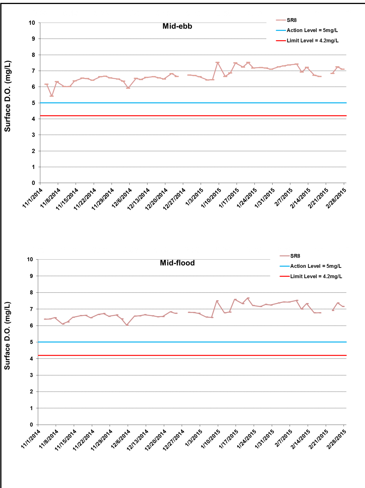
Figure G8 Impact Monitoring - Mean Level of Dissolved Oxygen (mg/L) in surface waters between 1 November 2014 and 28 February 2015 at SR8. The weather conditions during the monitoring period varied mostly from sunny to cloudy. Major marine construction activities included: Construction of Temporary Seawalls (11/1/2014 - 11/20/2014); Sheet Piling (11/1/2014 - 11/20/2014); Filling (11/1/2014 - 11/20/2014). WQM on 20 February 2015 was postponed to 23 February 2015. Ref: 0212330_Impact-WQM_February2015_graphs_Rev a.xls
