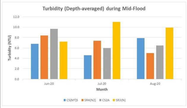
Figure G4 Operational Phase Monitoring - Mean Depth-averaged Level of Turbidity (NTU) between 1 June 2020 and 31 August 2020. The weather conditions during the monitoring period varied mostly from sunny to cloudy.
