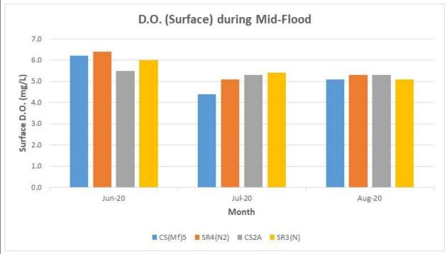
Figure G1 Operational Phase Monitoring - Mean Level of Dissolved Oxygen (mg/L) in surface waters between 1 June 2020 and 31 August 2020. The weather conditions during the monitoring period varied mostly from sunny to cloudy.
