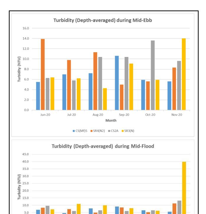
Figure G4 Operational Phase Monitoring – Mean Depth-averaged Level of Turbidity (NTU) between 1 June 2020 and 30 November 2020. The weather conditions during the monitoring period varied mostly from sunny to cloudy.
