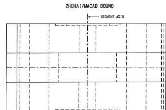
MONOLITHIC PIER AT NAVIGATION CHANNEL (APPLICABLE TO PIERS P82 AND P83) SCALE 1:100
